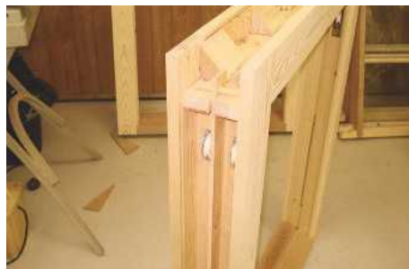
▲ Pic.27 The final move is to hang the wagtail in place and slide in the 6mm ply back
